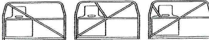
ADDITIONAL BRACING BEHIND DRIVER'S HEAD IN MAIN HOOP REQUIRED.
